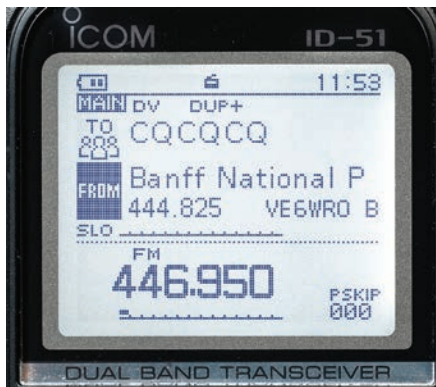
Figure 1 — Despite the size constraints of a handheld radio, the ID-51A's display resolution is high enough to show quite a bit of data clearly.
